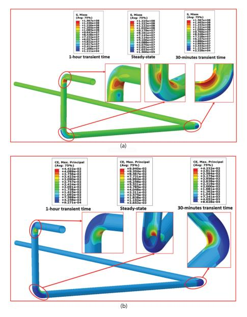
Figure 9: Creep (a) stress and (b) strain contour plot profile at failure
