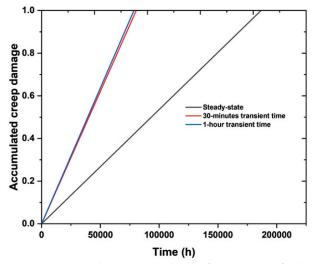
Figure 10: Creep damage accumulation of steam piping for the different cycles considered
