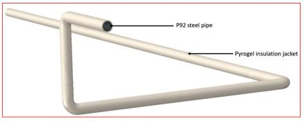
Figure 1: Assembly model of pipe-insulation jacket
