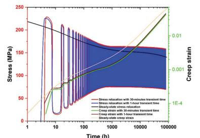
**Time (h) Figure 12:** Pattern for relaxation of stress and creep strain for different cycles of operation
