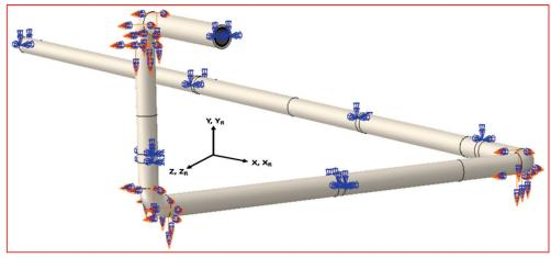
Figure 4: Applied boundary conditions on the assembly
