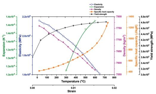
Figure 2: Thermal/mechanical properties of P92 steel (Salifu, et al., 2021a)
