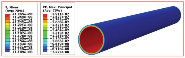
Figure 8: Developed creep stress and strain after one hour steady-state analysis in straight pipe
