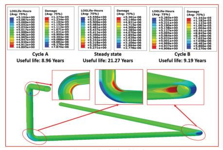
Figure 11: Steam piping creep damage and useful life at failure for operating cycles
