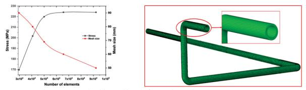
Figure 5: (a) Mesh convergence graph and (b) assembly mesh of pipe-insulation jacket
