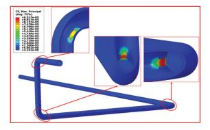
Figure 7: Steam piping creep (a) stress plot and (b) strain plot profile
