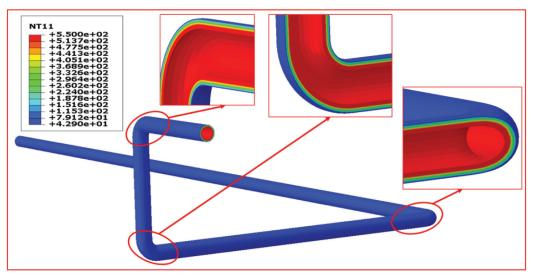
Figure 6: Steam piping temperature distribution profile in
