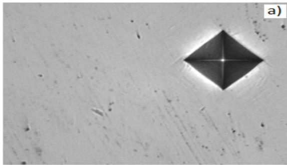
**Figure 3:** Micro-hardness indentation of the as-built
