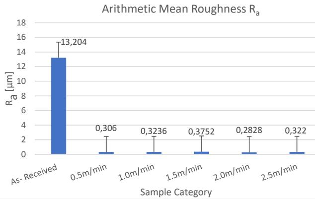
**Figure 7:** Average Ra and Standard Deviation of Laser Re-melted samples for varied Laser Scanning Speed
