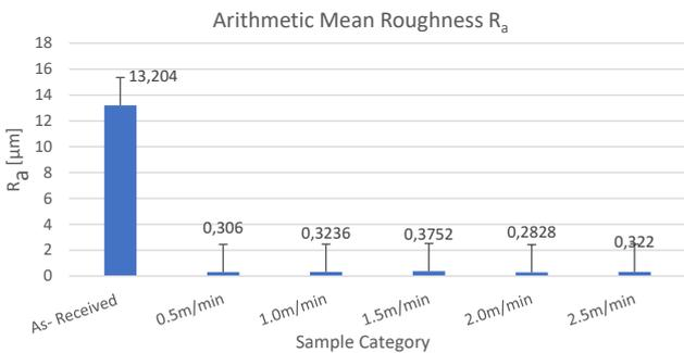
**Figure 8:** Average Ra and Standard Deviation of Laser Re-melted samples for varied Laser Scanning Speed
