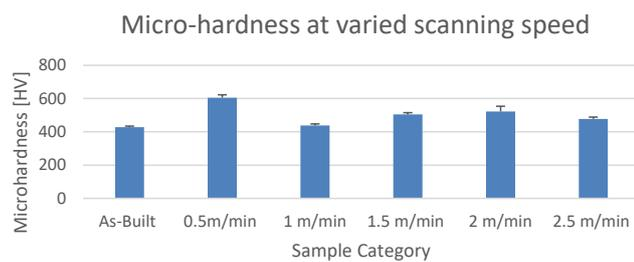
**Figure 4:** Micro-hardness test measures at different laser scanning speed
