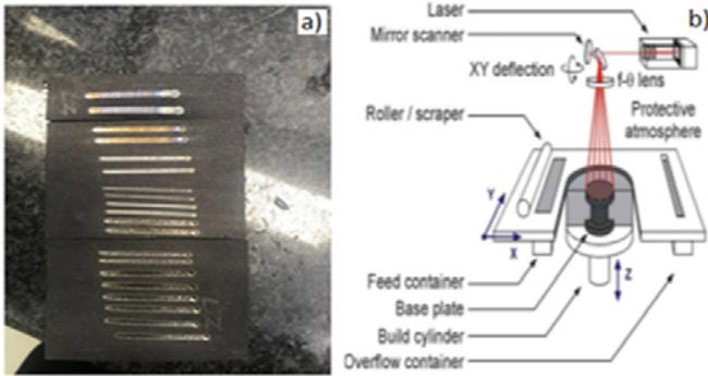
**Figure 1:** a) Test parts built by SLM and exposed to laser surface re-melting, b) Operating principle of SLM process Kruth et al. (2010)
