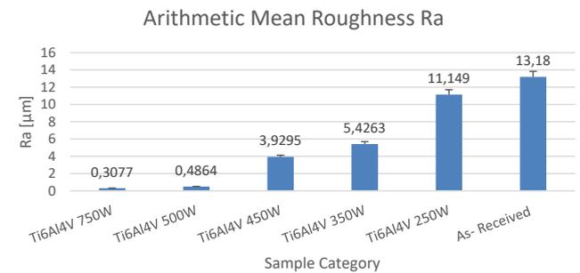
**Figure 6:** Average  $R_a$  and Standard Deviation of Laser Re-melted samples for varied Laser Power Outputs
