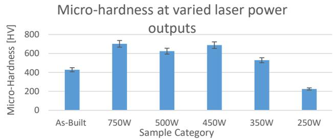
**Figure 5:** Micro-hardness test measures at different laser power outputs
