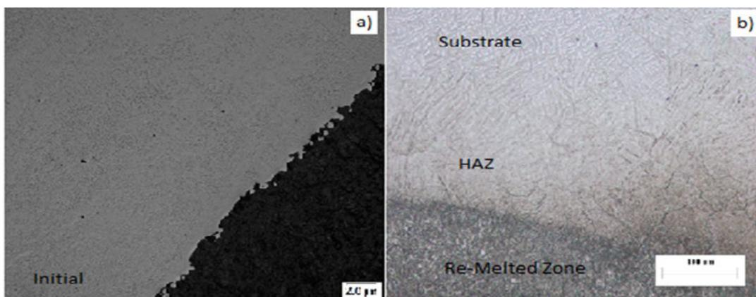
**Figure 2:** Re-melting trace cross section microstructure after LSR
